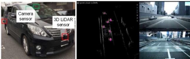
Fig. 4 An instrumented vehicle and a sample of real traffic data
